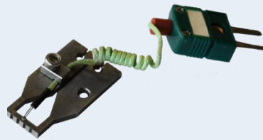
2D custom made thermode with thermocouple
