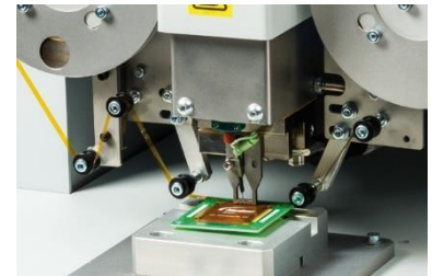
Soldering process with Kapton tape
