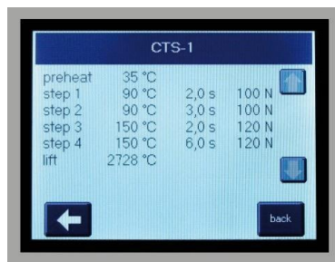
Steps screen. Each value in each step can be edited. The caption shows the name of the active program
