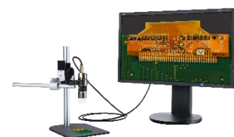
Step 5: product alignment control / quality inspection of the joint
