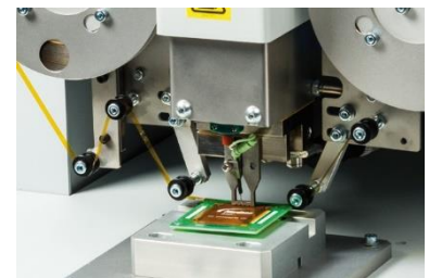
Soldering process with Kapton tape
